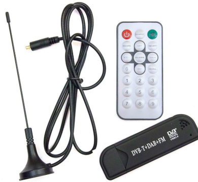
Figure 1. RTL-SDR hardware: USB DVB-T tuner based on RTL2832U chipset, made in China
